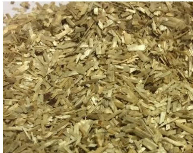
Figure 1. Crushed and sifted flax shives.
