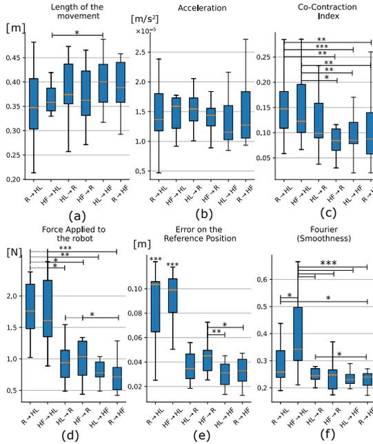
**Fig. 2** Comparison of the experimental conditions at the first 5 iterations after the switching: ( $M_1$ ) Length of the movement; ( $M_2$ ) Acceleration; ( $M_3$ ) Co-Contraction index of the subject and measured using EMG sensors; ( $M_4$ ) Force applied to the cobot; ( $M_5$ ) Error on the reference position; ( $M_6$ ) Fourier. The six experimental conditions are the combinations of the three control modes: Human Leader( $HL$ ), Human Follower( $HF$ ) and Reciprocal( $R$ ).
