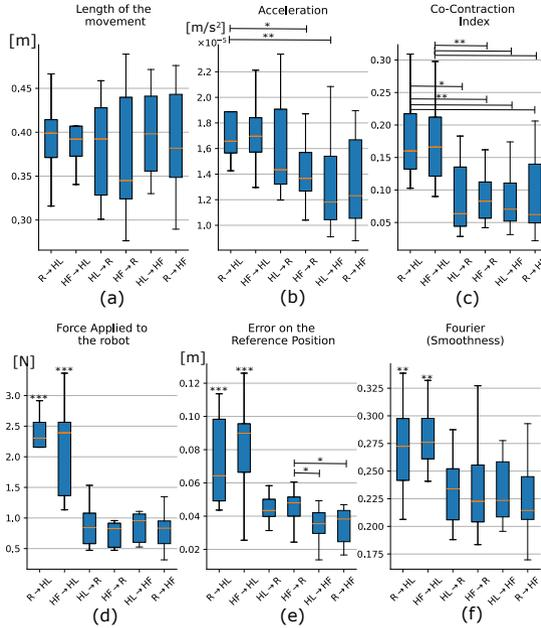
**Fig. 3** Comparison of the experimental conditions at Steady State: to identify steady state linear regressions were calculated for each of the six experimental conditions iteratively for the last 60, 59, 58 trials and so forth until the slopes were not significantly different from zero (i.e. the 95 % intervals did include zero).
