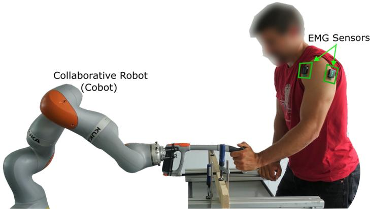
**Fig. 1** The experimental setup: the cobot is semi-rigidly attached to the saw, likewise the subject grabs the saw from the other end. EMG sensors are attached to the subject to measure muscle contraction during movement.
