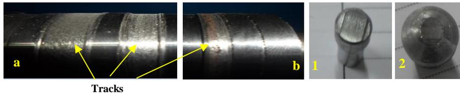
Figure 8. Cylinder and pins track after tribology: (a) and (1) Dry contact, (b) and (2) Lubricated contact
