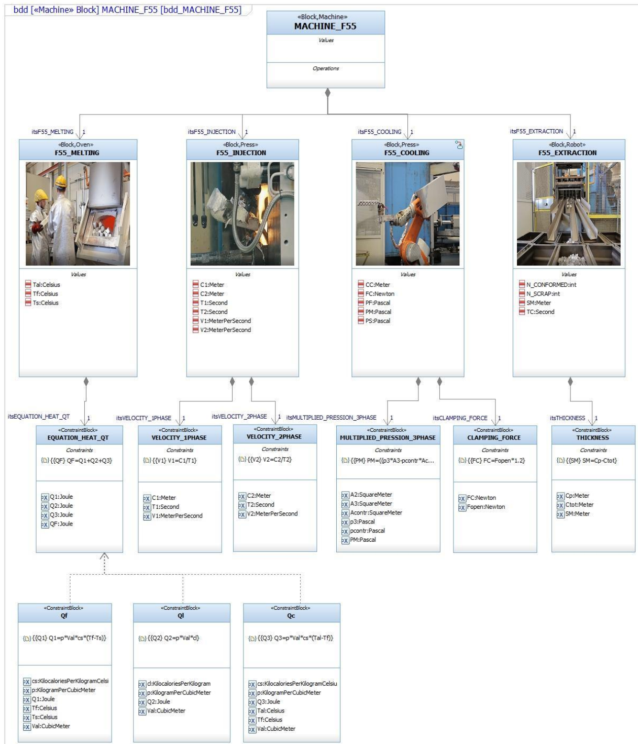
Figure 10: Block Definition Diagram of Die-casting Process (bdd)
