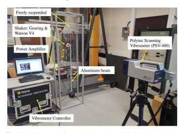
Fig. 16. Experiment set-up for measuring the vibratory field of the aluminum beam
