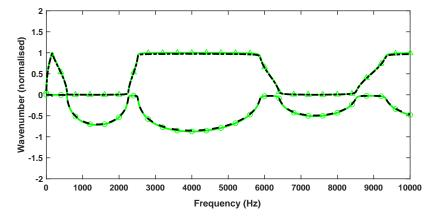
Fig. 15. Comparison of dispersion curves obtained by AWI and WFEM for a bi-material periodic beam under small perturbation condition when the unit-cell length is unknown. ( $\triangle$ —) real part of the wavenumber obtained by AWI, ( $\circ$ —) imaginary part of the wavenumber obtained by AWI, ( $\circ$ —) real part of the wavenumber obtained by WFEM, ( $\circ$ —) imaginary part of the wavenumber obtained by WFEM.
