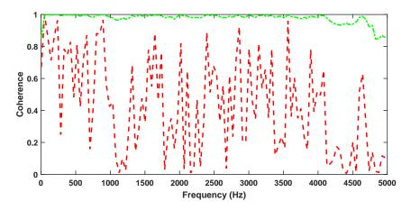
Fig. 17. Envelope of coherence function calculated for all measurement points. (- - -) minimum value of coherence function (---) maximum value of coherence function.
