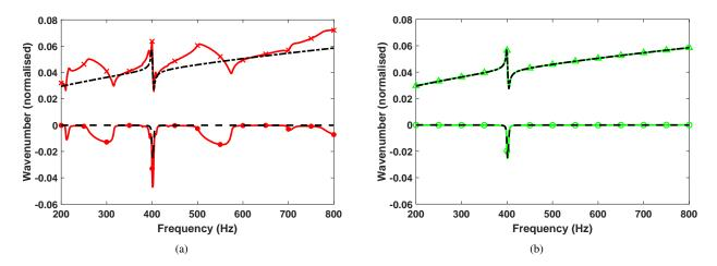
**Fig. 11.** Dispersion curves comparison for a homogeneous beam with TMDs under nonuniform sampling and small perturbation condition: (a) INCOME and WFEM; (b) AWI and WFEM. (★—) real part of the wavenumber obtained by INCOME, (♠—) imaginary part of the wavenumber obtained by AWI, (♠—) imaginary part of the wavenumber obtained by AWI, (♠—) real part of the wavenumber obtained by WFEM, (← - −) imaginary part of the wavenumber obtained by WFEM.
