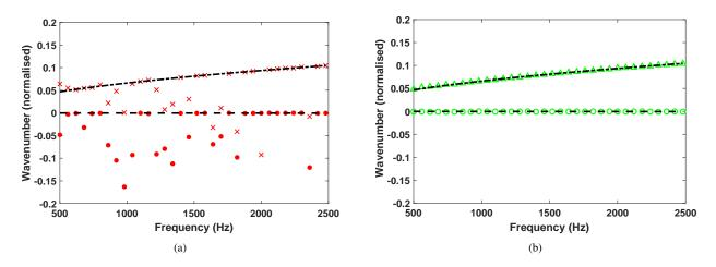
Fig. 6. Dispersion curves comparison for a homogeneous beam under signal noise (SNR=25) condition: (a) INCOME and WFEM; (b) AWI and WFEM. ( $\times$ ) real part of the wavenumber obtained by INCOME, ( $\bullet$ ) imaginary part of the wavenumber obtained by AWI, ( $\circ$ ) imaginary part of the wavenumber obtained by AWI, ( $\circ$ ) imaginary part of the wavenumber obtained by WFEM, ( $\circ$ ) imaginary part of the wavenumber obtained by WFEM.
