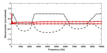
**Fig. 14.** Comparison of dispersion curves obtained by INCOME and WFEM for a bi-material periodic beam under the perfect condition when the unit-cell length is unknown. (**x**—) real part of the wavenumber obtained by INCOME, (•—) imaginary part of the wavenumber obtained by INCOME, (---) real part of the wavenumber obtained by WFEM, (---) imaginary part of the wavenumber obtained by WFEM.
