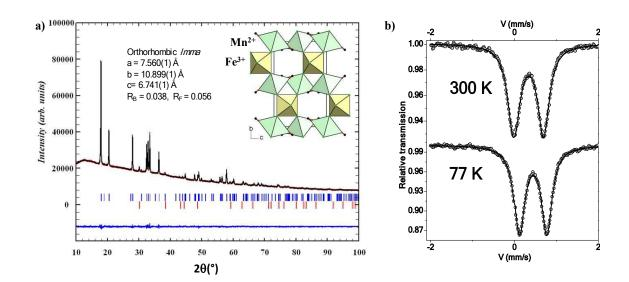
Figure 1. Final Rietveld profile refinement of X-ray powder diffraction pattern (a) and <sup>57</sup>Fe Mössbauer spectra at 300K and 77K (b) of MnFeF<sub>5</sub>(H<sub>2</sub>O)<sub>2</sub>.
