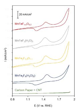
Figure 4: CVs of Mn-based fluorinated materials in 0.5 M H<sub>2</sub>SO<sub>4</sub> electrolyte at 20 mV/sec. scan rate.
