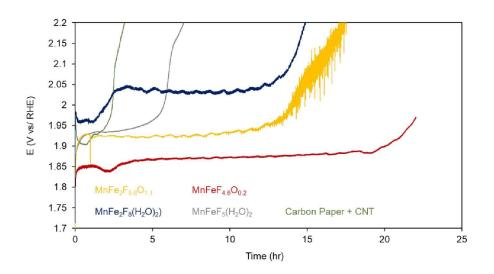
Figure 5 : Chronopotentiometric scans of each Mn material at 10 mA/cm<sup>2</sup> in 0.5 M H<sub>2</sub>SO<sub>4</sub> electrolyte.
