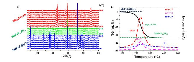
Figure 2. a) Thermal evolution of the X-ray diffractograms under air and b) TGA-MS analyses under N<sub>2</sub> of MnFeF<sub>5</sub>(H<sub>2</sub>O)<sub>2</sub>.
