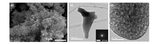
Figure 3: a) SEM and b) and c) TEM images of MnFeF<sub>4.6</sub>O<sub>0.2</sub> obtained after calcination of MnFeF<sub>5</sub>(H<sub>2</sub>O)<sub>2.</sub> Inset of b): Corresponding SAED.
