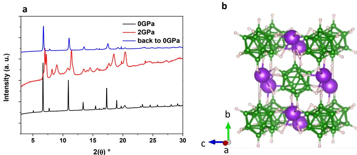
**Figure 2.** Diffraction patterns of  $\text{K}_2\text{B}_{12}\text{H}_{12}$  at 0 GPa (black), 2 GPa (red) and back to ambient pressure (blue) depicting it reversible pressure induced phase transition (a). Representation of the  $\text{hp}\text{-}\beta\text{-K}_2\text{B}_{12}\text{H}_{12}$  crystal structure (b).
