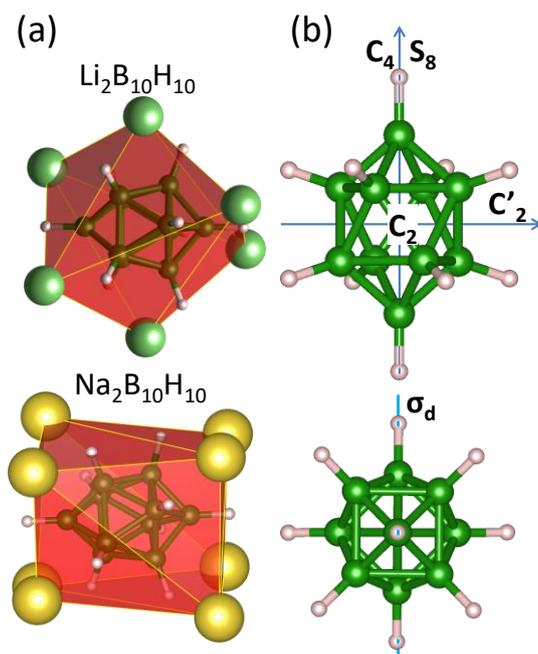
**Figure 7.** Coordination polyhedra for  $B_{10}H_{10}^{2-}$  anions in alkali metal deca H-c-B. Small green/gray spheres are for boron/hydrogen; large green are Li, yellow – Na (a). The schematic view of the symmetry elements of  $D_{4d}$  point group of  $B_{10}H_{10}^{2-}$  anion:  $C_4/S_8$  are rotations/improper rotations around four-fold and eight-fold axis,  $C_2/C'_2$  are rotations around two-fold axis, and  $\sigma_d$  stands for the mirror plane (b).
