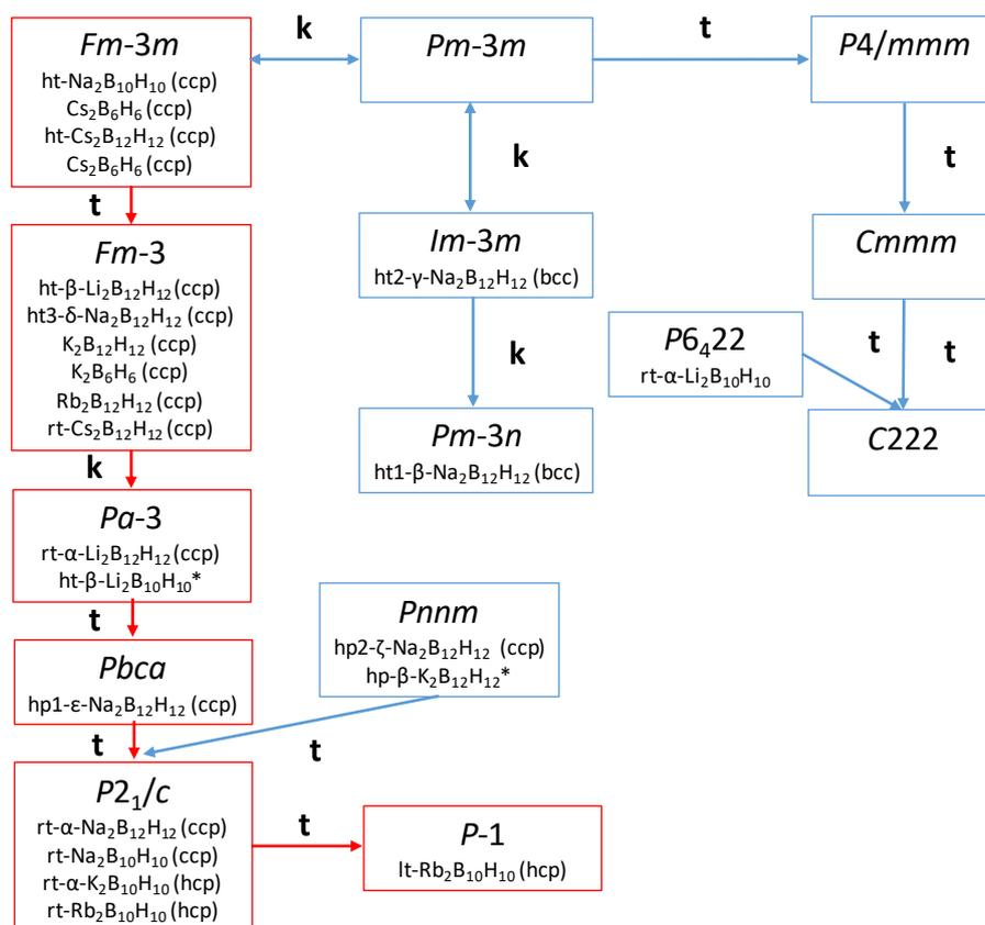
**Figure 1.** Group-subgroup relationship between the hydrido-closo-borates. t stands for *translationengleich* and k *klassengleich* subgroups. The asterisk \* indicates the crystal structures determined in this work. rt and lt stand for room temperature and low temperature, here below 250 K, respectively.
