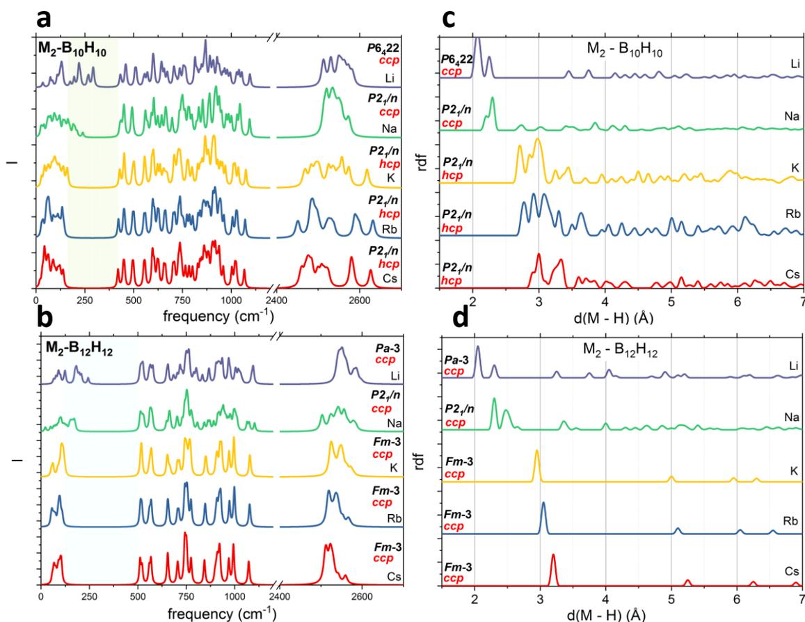
**Figure 6.** Distribution of the phonon distribution at the  $\Gamma$ -point for alkali metal deca H-*c*-B (a) and dodeca H-*c*-B (b), and the radial distribution function for cation – hydrogen separation for alkali metal deca H-*c*-B (c) and dodeca H-*c*-B (d). The calculated frequencies are broadened with 5  $cm^{-1}$  Lorentzian.
