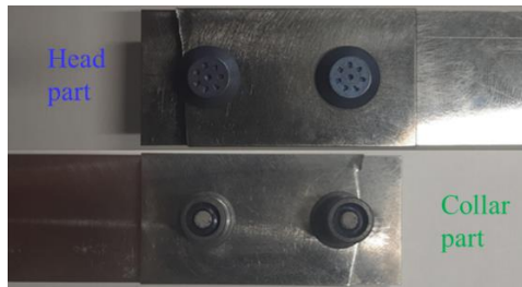
Fig. 5. Fatigue failure locations, head side on the upper picture, collar side on the lower picture
