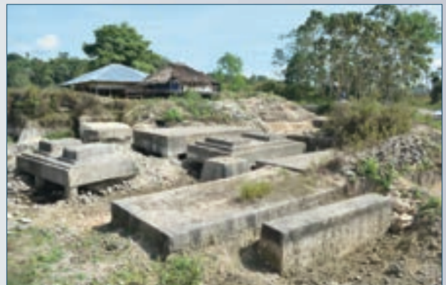
Fig. 3 – Quarry in Anakalang district. Chambers and capstones are waiting to be extracted (Photos: N. Bec Drelon).
