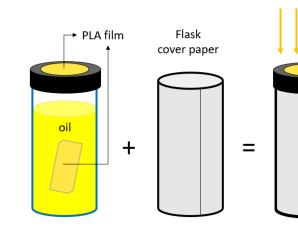
Vials with Exchange surface of 3 cm<sup>2</sup> were placed under white lamps (4700  $\pm$ 200 lux) at RT. The peroxide value (PV) of the oil samples was periodically determined according to the IUPAC titration method for oils, fats and derivatives oils.
