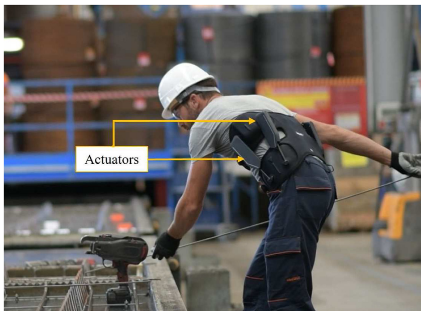
Figure 2. Japet. W following the inclination of the trunk.
