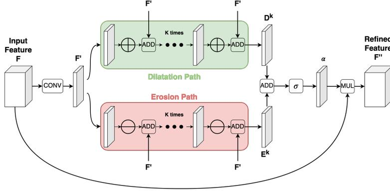
Figure 2: Diagram of proposed Morphological Attention Gate
