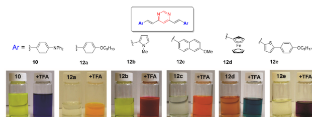
Fig. 7 Digital photographs showing the color change experienced by CH_2Cl_2 solutions of various bis(arylviny)pyrimidines 10 and 12 in the presence of 10^{-2} M TFA. Adapted from ref. 14, (copyright 2009, American chemical Society).
