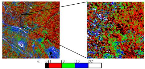
Fig. 2: Detail of the ground point density map; the color corresponds to the number d of points per pixel (1 m<sup>2</sup>).
