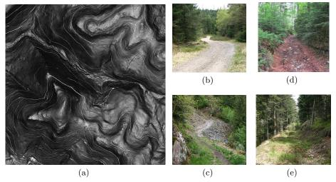
Fig. 1: (a) A shaded digital terrain model (DTM) image of size  $4000 \times 4000$  pixels and  $0.25 \text{ m}^2/\text{pixel}$  resolution, that corresponds to a  $4 \text{ km}^2$  area. (b–e) Different forest road types in mountainous context: (b) logging road with large vegetated shoulders at the same height, (c) shrinked road crossing natural screes, (d) eroded hollow road, and (e) unused road left to growing vegetation.
