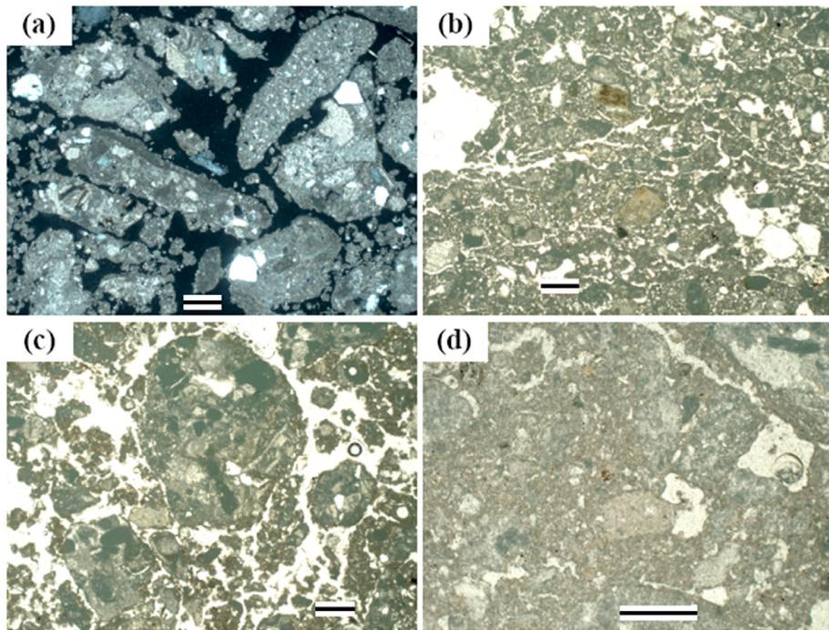
**Fig. 8.** Photomicrographs of primary microfacies types (scale 500 µm) (a) MF type 1 (b) MF type 2 (c) MF Type 3 (d) MF Type 4.
