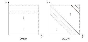
Fig. 1. Variation in frequency (Y axis) of the data symbols subcarriers in function of the time (X axis) in OFDM (sinusoids) and OCDM (chirps).
