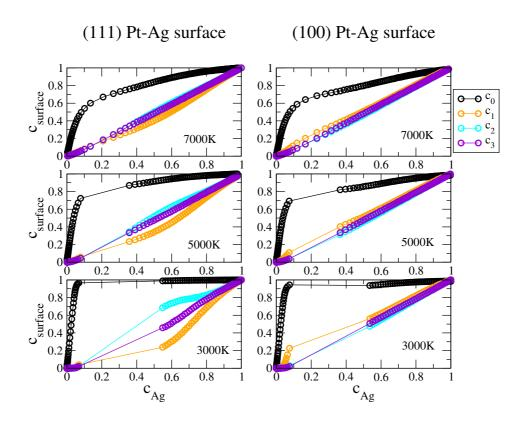
FIG. 8. Segregation isotherms at (111) and (100) surfaces at 7000K, 5000K and 3000K where we plot the top surface  $c_0$ , the subsurface  $c_1$  and the following  $c_2$  and  $c_3$  atomic layers concentrations in silver by increasing (up) or decreasing (down) the chemical potential.
