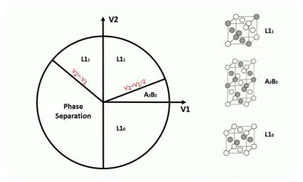
FIG. 1. Ground state diagram of an Ising model for Effective Pair Interactions (EPIs) on fcc lattice at first and second neighbors [12, 23, 27].
