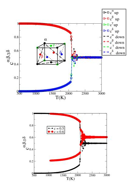
FIG. 5. Bulk sublattices from canonical Monte Carlo simulations at equiconcentration (top graph) and c=0.6 (bottom graph) with increasing (up) and decreasing (down) temperature. The sublattices are defined relatively to the (111) cristallographic planes. The L1<sub>1</sub> phase is characterized by the sublattices occupied two by two by Ag or Pt atoms. The disordered A1 solid solution is characterized by the four sublattices equally occupied.
