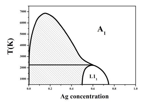
FIG. 7. Theoretical bulk phase diagram with the TBIM model and variable EPIs.
