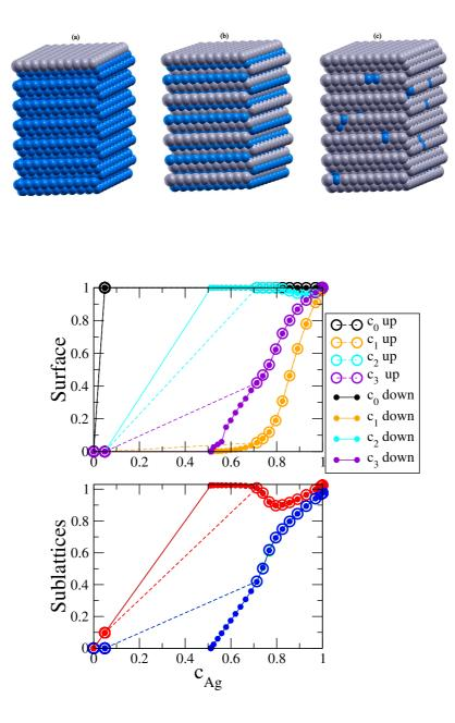
FIG. 9. Segregation isotherms of the (111) surface at 300 K. The slabs are illustrated on top for three characteristic concentrations (a) below 5%, (b) 50% and (c) above 80% with Ag atoms in grey and Pt atoms in blue. Then the first four layers concentrations starting from the surface  $c_0$ ,  $c_1$ ,  $c_2$  and  $c_3$  are plotted in the top graph and finally the core sublattices concentrations are plotted in the bottom graph as a function of the global Ag concentration.
