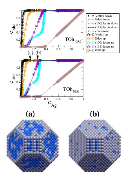
FIG. 13. Segregation isotherms of  $TOh_{1289}$  and  $TOh_{2951}$  cluster at 1000 K for each different surface sites (vertex, edge, (111) and (100) facets) and core sites, and for up and down simulations (which are superimposed) with the same symbols as for the surfaces. Illustration of the  $TOh_{2951}$  cluster at 5% (a) and 25% (b) of Ag.
