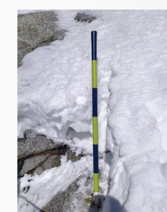
Figure 3C: Snow depth measurement pole
