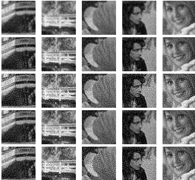
Figure 12: Samples from example 8.5. From top to bottom: noisy image, reconstruction with vanilla 3D having access to the GTG (i.e. x_{\bar{n}} ), reconstruction with vanilla 3D using SURE (i.e. x_{\hat{n}} ), and reconstruction with warm 3D ( x_{\bar{n}} then x_{\hat{n}} ).
