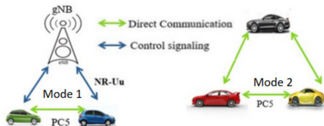
Fig. 1: Resource Allocation Modes in 5G-V2X
