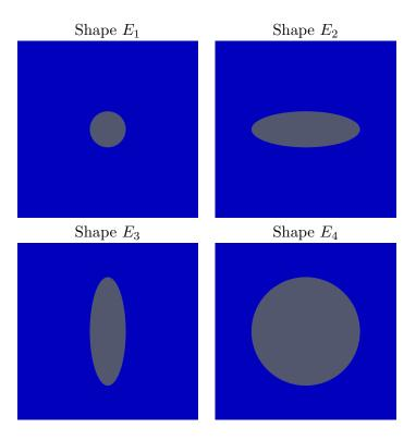
Figure 4: Representation of the 2D reference cells Y' used in the numerical simulations of the effective models. The inclusion T' (in grey) is surrounded by  $Y'_f$  (in blue). From left to right and top to bottom: disk or radius 0.1, ellipses of semi-major axis 0.3 and semi-minor axis 0.1, oriented respectively along the x and y directions, and disk of radius 0.3. These shapes are numbered  $E_1, E_2, E_3$  and  $E_4$ .
