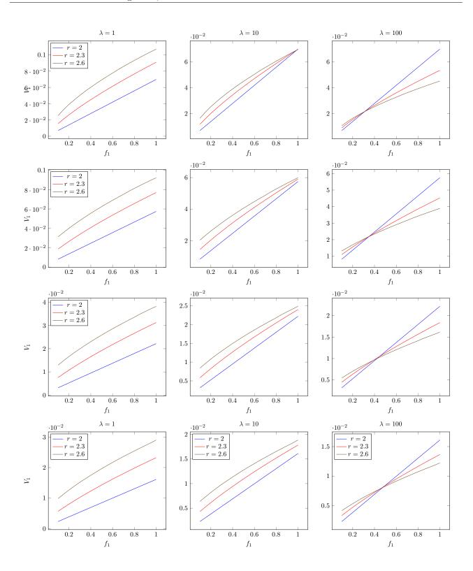
Figure 9: Case  $\gamma > 1$ , r > 1 (power law). Component  $V_1$  of the mean filtration velocity V' plotted against  $f_1$ , with  $f' = (f_1, 0)$ , for  $r \in \{2, 2.3, 2.6\}$  and elliptic inclusions  $E_1$  (first line),  $E_2$  (second line),  $E_3$  (third line) and  $E_4$  (fourth line). From left to right:  $\lambda = 1, \lambda = 10, \lambda = 100$ .
