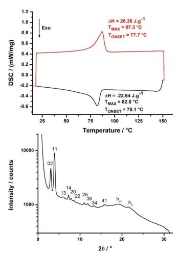
Figure 3. (Top) DSC trace of compound 2 (Top:  $2^{nd}$  heating curve; bottom:  $1^{st}$  cooling curve). (Bottom) SAXS pattern of compound 2 at 150 °C (second heating) with peak indexation.
