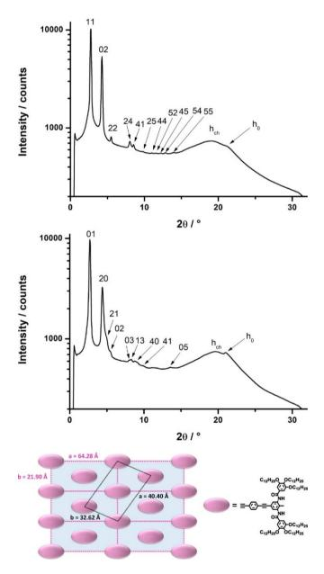
**Figure 2.** SAXS pattern after second heating of compound 1 at 170 °C (Top), at 100 °C (Middle) ((hk) indexation,  $h_{ch}$ : maximum of the diffuse scattering due to lateral distances between molten aliphatic tails,  $h_0$ : diffuse scattering due to  $\pi$ - $\pi$  stacking. (Bottom) Schematics of the rectangular (pink) and oblique (black) unit cell found at 170 °C and 100 °C, respectively.
