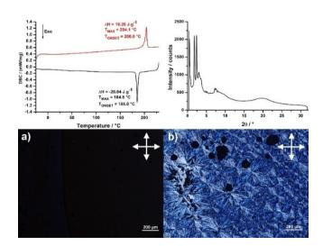
**Figure 5.** (Top left) DSC trace of **Ru**<sub>2</sub> (Top: 2nd heating curve; bottom: 1st cooling curve). (Top right) SAXS pattern of **Ru**<sub>2</sub> at 150 °C (second heating). (Bottom) a) POM image of **Ru**<sub>2</sub> at 180 °C and b) at 173 °C after cooling from the isotropic state (crossed-polarizers symbolized by the white cross in the corner of the picture).
