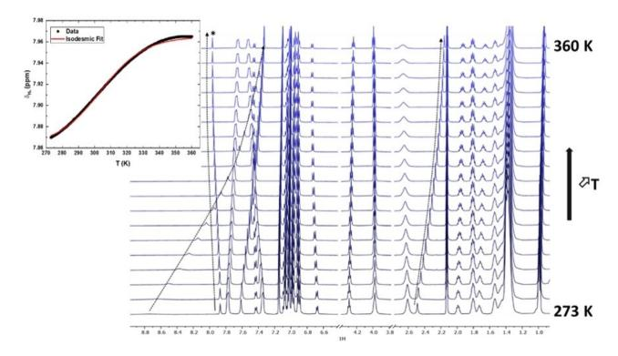
Figure 6. VT-<sup>1</sup>H NMR monitoring of a 10 mM solution of Ru<sub>2</sub> in toluene-d<sub>8</sub>. (Inset) Plotting of the chemical shift variation of the singlet signal marked with a (\*) as a function of the temperature.
