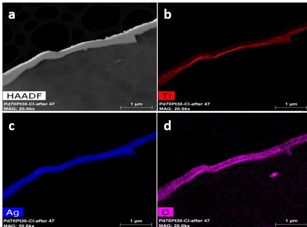
**Figure 2.** TEM images of  $\text{Ag}_x\text{O-TiO}_2\text{-PES}$  as sputtered by HiPIMS at a current of 30 A for 20s: a) High-angle annular dark-field imaging (HAADF), b) EDXS mapping of Ti, c) EDXS mapping of Ag, and d) EDXS mapping of O.
