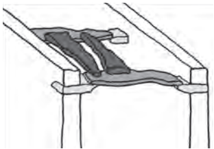
35. The three structural levels of the stone roof in the fort: corbels (light grey) support lintels (mid-grey), supporting in turn another level of lintels (dark grey) (Q. Devers, 2012).
