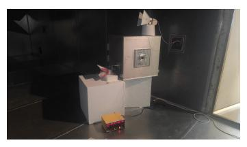
Fig. 5. View of the experimental setup installed in the large RC. The Faraday cage is shown with the source antenna on the top and the receiving antenna on its left side. The front size contains the windows where the screen is inserted for SE measurements
