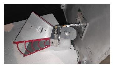
Fig. 6. Detection antenna, low noise amplifier and rectifier outside the Faraday cage
