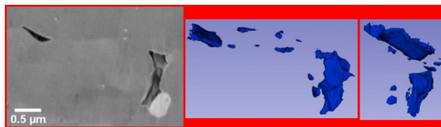
Figure 16: Std-63 at OR, detailed image on intergranular bubbles and associated 3D views showing that these bubbles, small or large, are closed, even that on grain edges (on the right on the micrograph and on the first 3D view)
