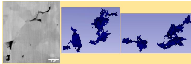
Figure 20: Std-73 at 0.35R, detailed image on intergranular bubbles and associated 3D views showing that these bubbles are complex but closed, even on grain edges
