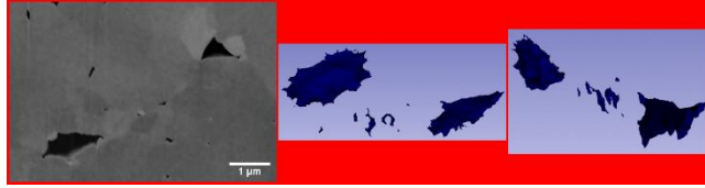
Figure 17: Std-73 at OR, detailed image on intergranular bubbles and associated 3D views showing that these bubbles, small or large, are closed, even that on grain edges (on the right on the micrograph and on the 3D views)
