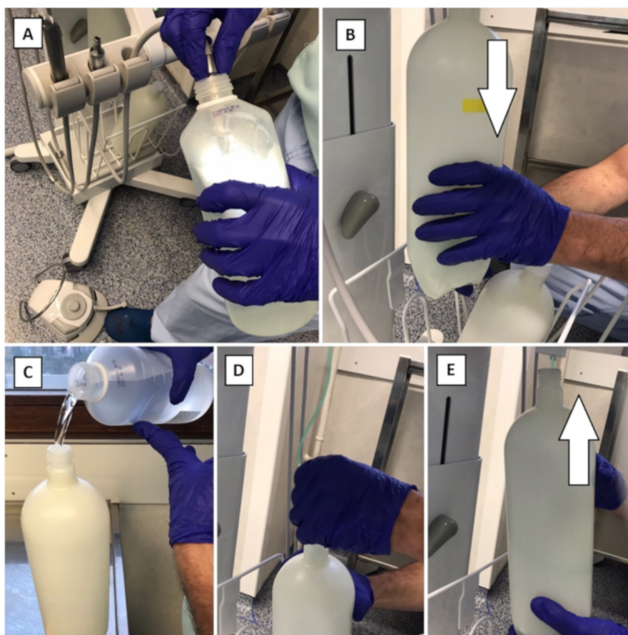
Figure 3. Parts of the maintenance protocol of the mobile dental delivery system (MDDS), before use and between each patient. (A) Purge of the air/water spray and the handpieces hoses with the Calbenium© solution; (B) removal of the reservoir that contains the Calbenium© solution; (C) filling of another reservoir with sterile water; (D,E) placement of the reservoir containing sterile water.
