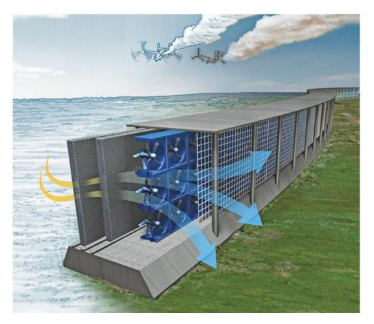
**Figure 4:** A hypothetical industrial DAC device with added photocatalyst, proposed to oxidize CH<sub>4</sub> into CO<sub>2</sub> [57]. Reproduced from John Bradley [82].
