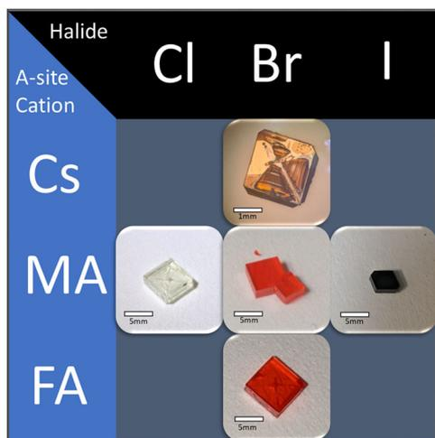
**Fig. 1 Pb-based HaP single crystals used in this study.** Horizontally:  $\text{MAPbX}_3$  ( $X = \text{Cl}, \text{Br}, \text{and I}$ ); vertically:  $\text{APbBr}_3$  ( $A = \text{Cs}, \text{MA}, \text{and FA}$ ).
