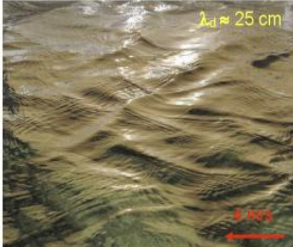
c) Dominant gravity waves ( \lambda \approx 25 \text{ cm} ) with capillaries at the crest wavefront observed at 4.0 \text{ m/s} wind speed.
