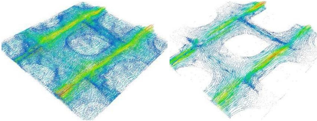
Fig. 5 Speed field from FE calculation with (left) and without Brinkman medium
