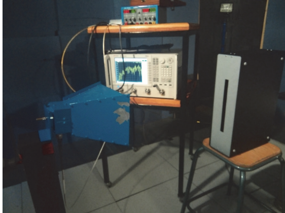
Fig. 6 – Measuring bench in semi-anechoic room.
