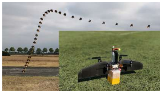
Figure 1: Sequential imagery of vertical take-off and transition of the finalized prototype with a close-up picture.
