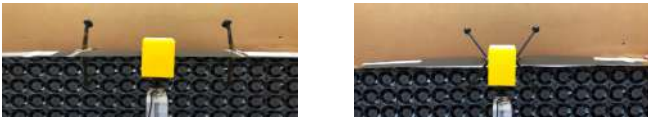
(a) Mounting arms in "H" (b) Mounting arms in "X" Figure 14: Test setup for arm configuration study. Half of the WindShape test section was covered to ease the visualisation.
