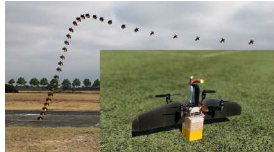
Figure 1: Sequential imagery of vertical take-off and transition of the finalized prototype with a close-up picture.
