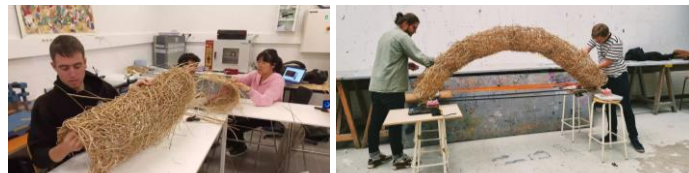
Figure 16: Braiding and loading tests on the 1:5 model.
