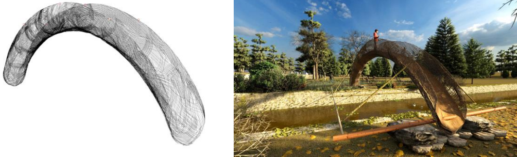
Figure 13: Optimal braiding of the bridge according to BAYA (the real diameter and number of strands have been reduced for a better reading) and corresponding 3D insertion (with the anti-buckling bamboos).
