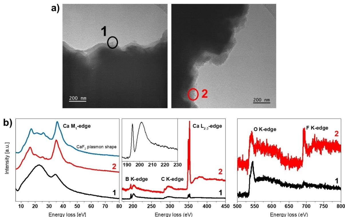
**Figure 4.** a) TEM of passivated nickel particles at a polarization potential of  $-4.0$  V vs.  $\text{Ag}_{\text{QRE}}$  during 48 h. b) The associated normalized EELS spectra corresponding to two different areas designated 1 and 2. Spectra normalized by the maximum intensity of signal for plasmon spectra, and the maximum intensity of B K-edge and O K-edge.
