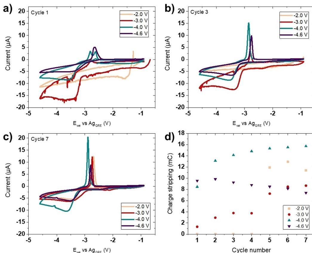
**Figure 1.** Cyclic voltammograms ( $0.4 \text{ mol L}^{-1} \text{ Ca(TFSI)}_2$  in EC:PC with 2 wt% of  $\text{BF}_3 \cdot \text{DE}$ ,  $0.1 \text{ mVs}^{-1}$ ,  $100^\circ\text{C}$ ) after 48 h potentiostatic polarization at  $-2.0 \text{ V}$ ,  $-3.0 \text{ V}$ ,  $-4.0 \text{ V}$  and  $-4.6 \text{ V}$  vs.  $\text{Ag}_{\text{QRE}}$ : a) cycle 1, b) cycle 3, c) cycle 7 and d) the charge stripping upon cycling.
