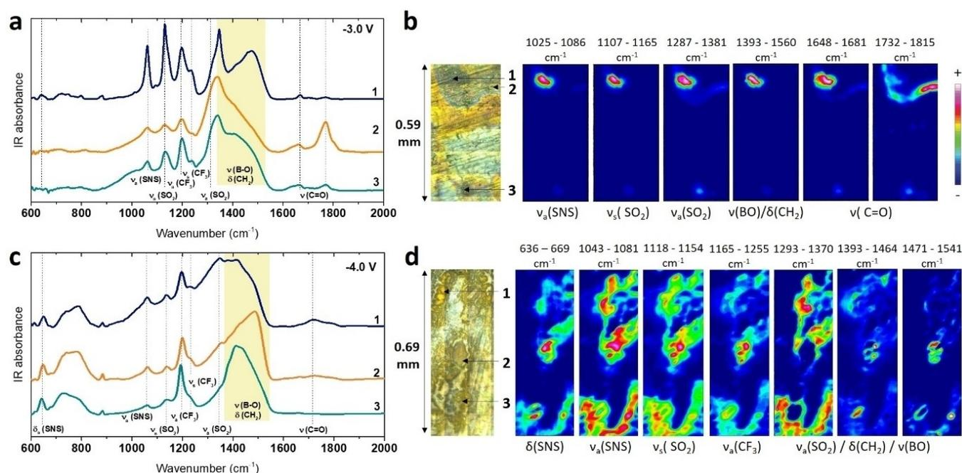
**Figure 6.** IR analysis of the SEI layers for the samples polarized during 48 h at a, b)  $-3.0$  V and c, d)  $-4.0$  V vs.  $\text{Ag}_{\text{QRE}}$ . a, c) FTIR-microspectroscopy spectra of the regions 1, 2, 3 marked on panels (b) and (d), dash lines are guides for the eye. b, d) Associated chemical images of the surface of the deposit for particular bands. The color scale corresponds to the intensity of the respective FTIR peak.
