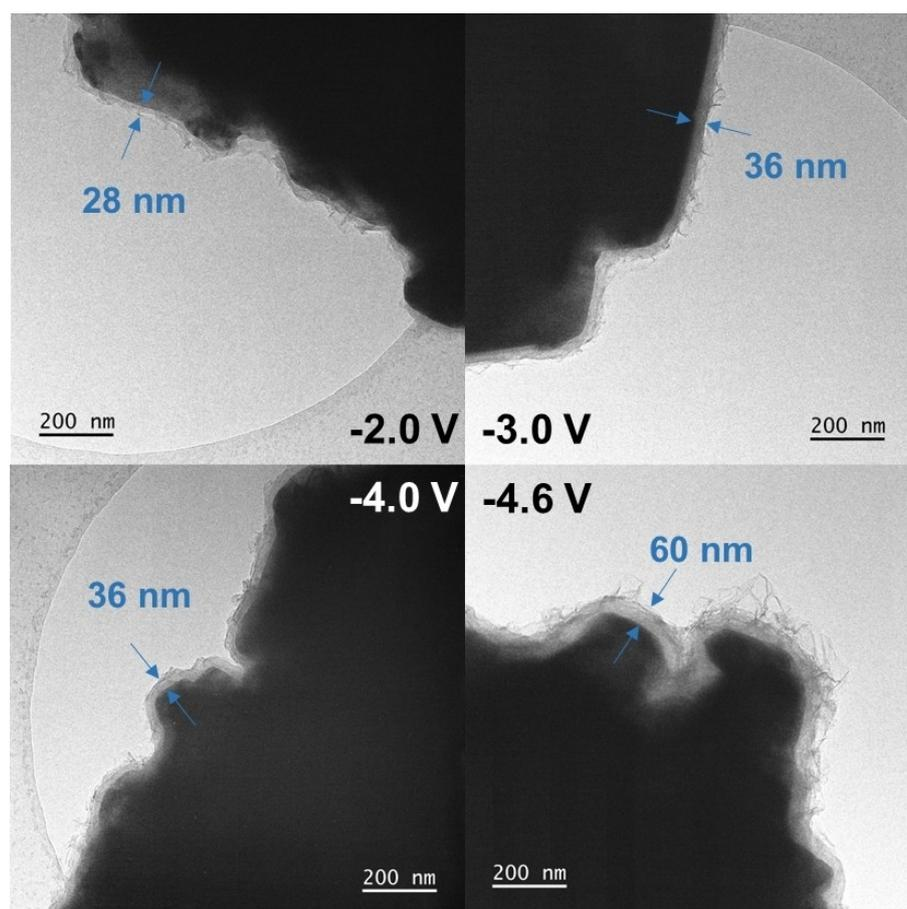
**Figure 3.** TEM images of passivation layer covered nickel particles prepared at  $-2.0$  V,  $-3.0$  V,  $-4.0$  V and  $-4.6$  V vs.  $\text{Ag}_{\text{QRE}}$  for 48 h at  $100^\circ\text{C}$  with  $0.4 \text{ mol L}^{-1}$   $\text{Ca}(\text{TFSI})_2$  in EC:PC + 2 wt% of  $\text{BF}_3 \cdot \text{DE}$  electrolyte.
