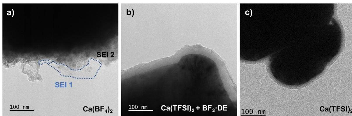
**Figure 2.** TEM images of passivated nickel particles polarized at  $100^\circ\text{C}$  for 48 h at a)  $-3.8 \text{ V}$ , and b and c)  $-4.0 \text{ V}$  vs.  $\text{Ag}_{\text{QRE}}$  with an electrolyte composed of a)  $0.5 \text{ mol L}^{-1} \text{ Ca(BF}_4)_2$  in EC:PC and b)  $0.4 \text{ mol L}^{-1} \text{ Ca(TFSI)}_2$  in EC:PC with 2 wt% of  $\text{BF}_3 \cdot \text{DE}$  or c) without.
