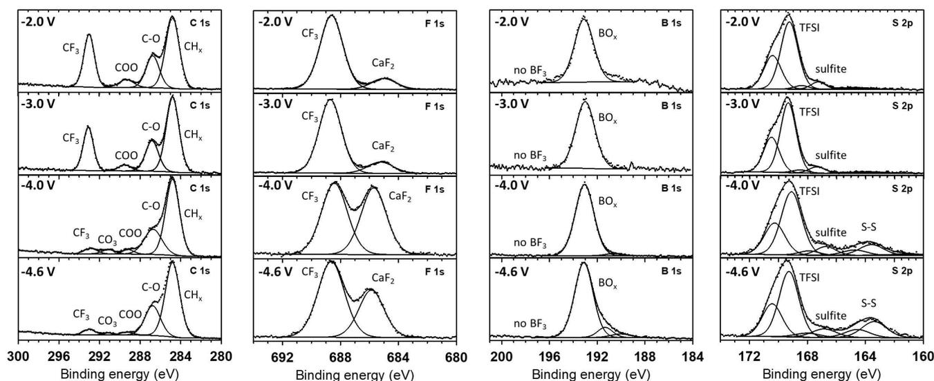
**Figure 5.** C 1s, F 1s, B 1s and S 2p XPS spectra of the surface layer deposited on nickel disks at different potentials (vs.  $Ag_{QRE}$ ). All disks were polarized for 48 h at 100 °C. Spectra are normalized by the most intense contribution.
