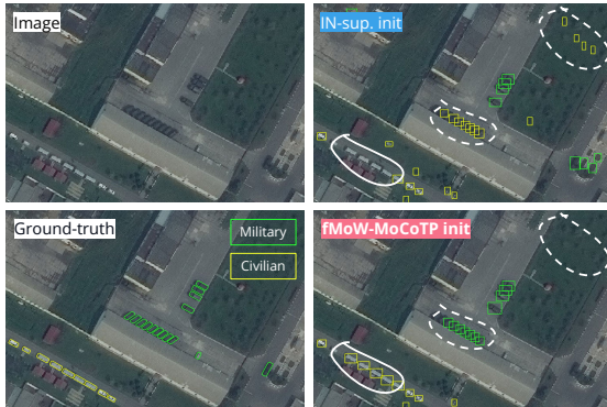
Fig. 3. Example of cherry-picked predictions. Here the models have been finetuned on an XS dataset. White regions highlights errors specific to the top model, in solid and dotted style for false negatives and false positives respectively.
