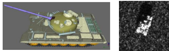
Figure 3. CAD model (left) and synthetic image example (right) of the T72.
