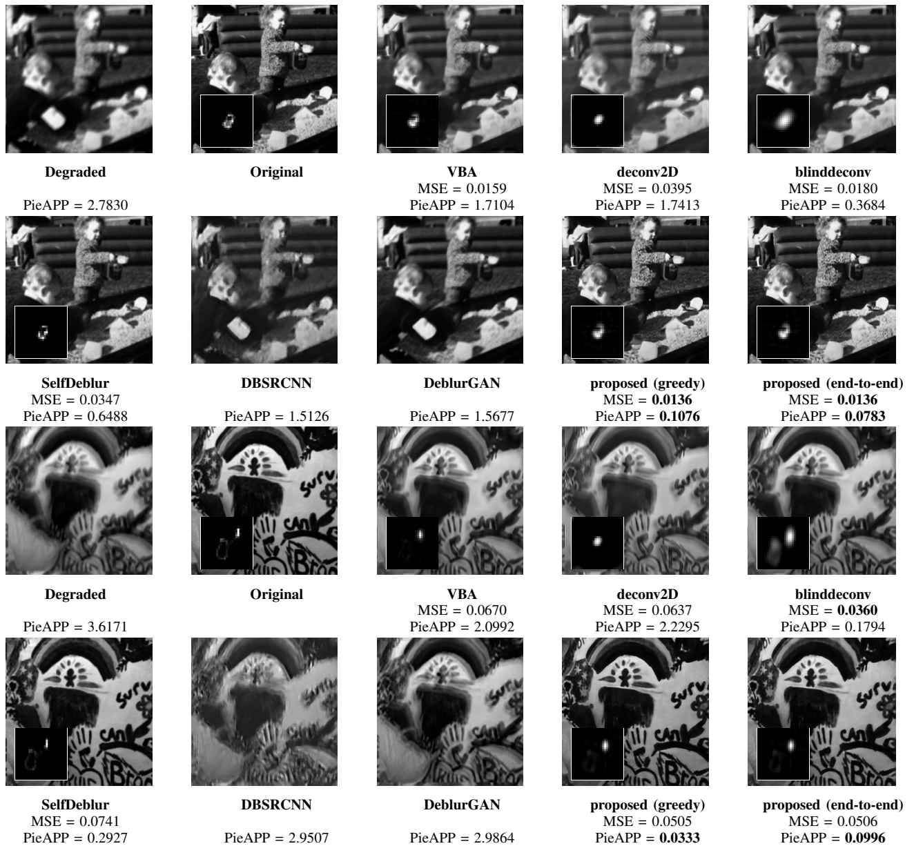
Fig. 10. Ground-truth image/blur, degraded image, restored images (with PicAPP index) and estimated blurs (with MSE score) when available, for various methods, on two examples in the test set of Dataset 3 .
