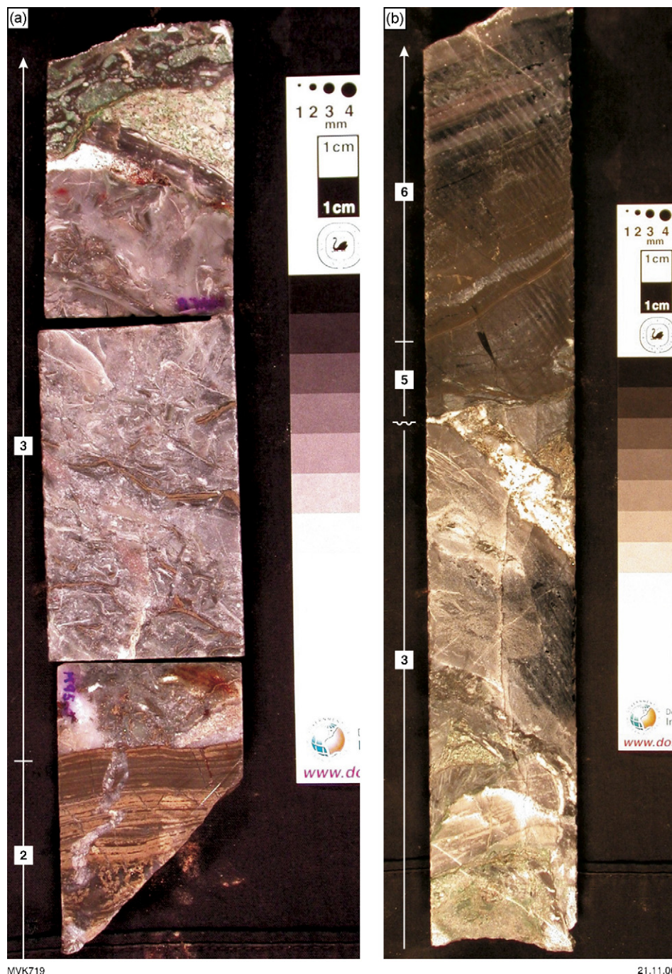
Fig. 10. Section of drillcore PDP2c, from 94.65 to 95.05 m depth: (a) lower half, showing pyritic laminates of member 2 at base, and lower part of diamictite of member 3; (b) upper half, showing upper part of diamictite of member 3, unconformably overlying basal conglomerate of member 5, and bedded carbonates of member 6 that are partly replaced by pyrite. Note the white carbonate–pyrite vein in member 3 that is cut off by the unconformity at the base of member 5.
