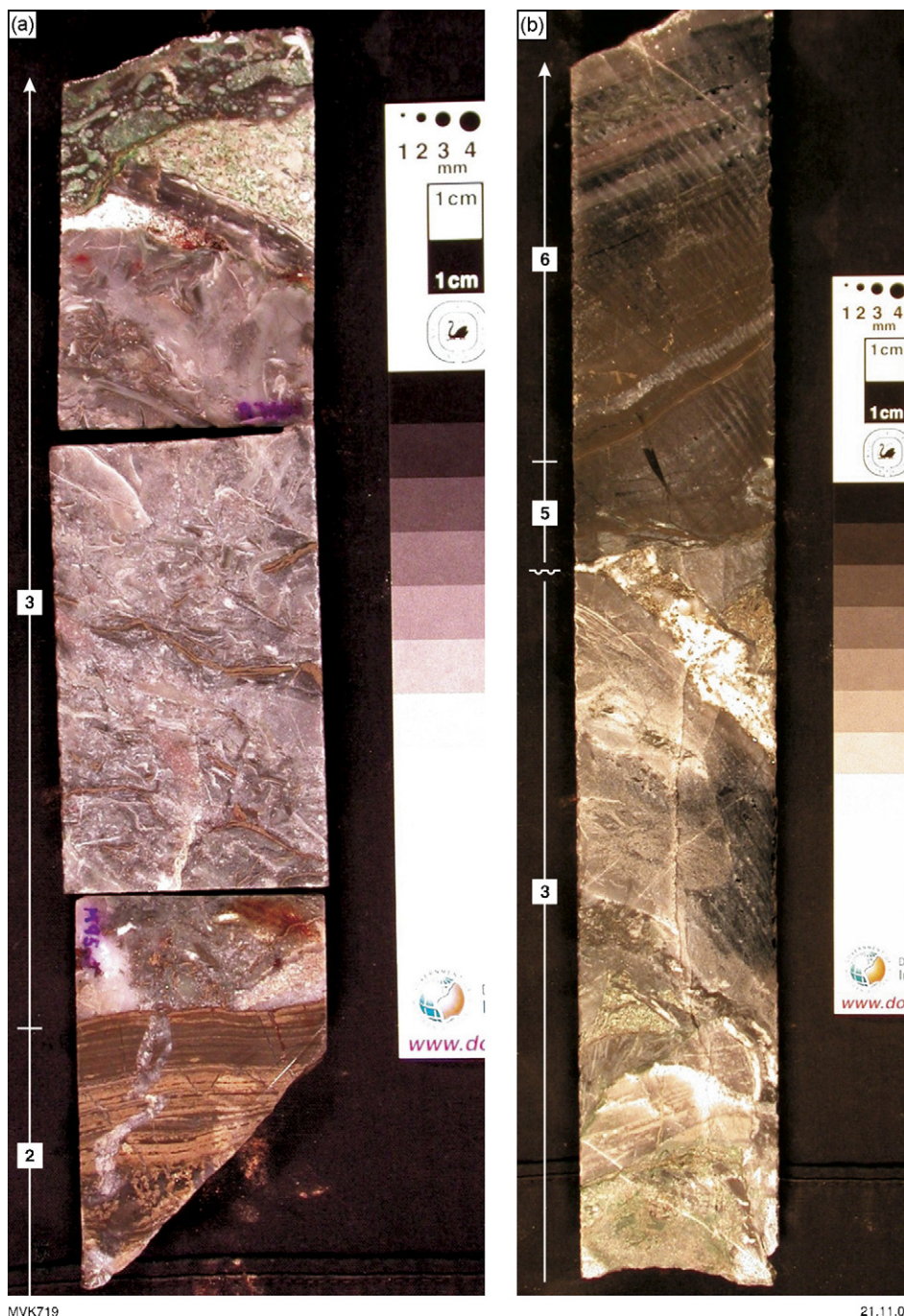
Fig. 10. Section of drillcore PDP2c, from 94.65 to 95.05 m depth: (a) lower half, showing pyritic laminates of member 2 at base, and lower part of diamictite of member 3; (b) upper half, showing upper part of diamictite of member 3, unconformably overlying basal conglomerate of member 5, and bedded carbonates of member 6 that are partly replaced by pyrite. Note the white carbonate–pyrite vein in member 3 that is cut off by the unconformity at the base of member 5.
