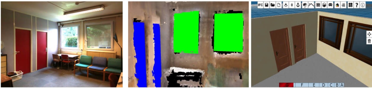
Figure 7. A 3D model viewed in the software Plan 3D Energy .
