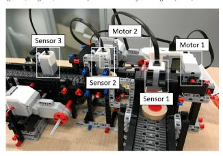
Fig. 1: basic elements of a station in a LEGO Manufacturing System. Sensor 1 detects if a part is queuing at the entrance of the station. Motor 1 lets the parts enter the station one at the time. Motor 2 drives the parts in the station and Sensor 2 detects if a part has entered. Sensor 3 detects if the downstream conveyor has enough slots for the parts to be released.
