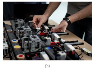
Fig. 3: two projects realized in the course: (a) buffer system allowing load/unload of pallets; (b) manufacturing system with three parallel stations.
