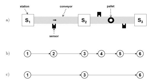
Figure 1: Problem introduction - (a) Three-station production line; (b) graph model with six nodes; (c) graph model with three nodes.
