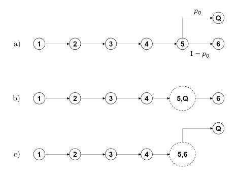
Figure 5: Test Case 2 – a) flow line graph model with six stations and a quality control station; b) graph model obtained with  $p_Q < 0.5$  and  $S_N^{max} = 6$ ; c) graph model obtained with  $p_Q \ge 0.5$  and  $S_N^{max} = 6$ .
