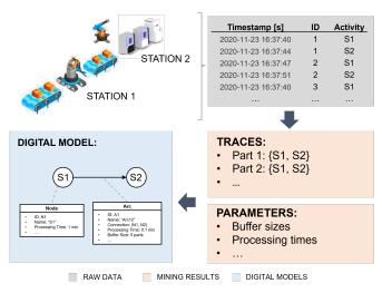
Fig. 3. Automated development of a material flow model.
