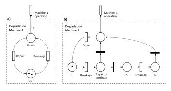
Fig. 5. Two exemplary Petri nets for machine degradation modeling.
