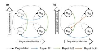
Fig. 4. State transition diagrams for joint machine degradation and maintenance policy modeling.
