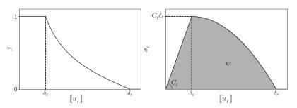
FIGURE 5. The form of cohesive law applied. On the left: evolution of the damage according to the normal/tangent displacement discontinuity. On the right: cohesive stress associated with a normal/tangent displacement jump [5].
