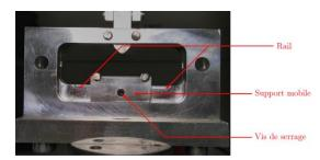
FIGURE 2. Design of the modular three-point flexion bench [3].
