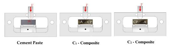
FIGURE 3. Geometry and boundary conditioned of samples subjected to three-point bending test (CP: Cement Paste and A: Aggregate).
