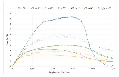
FIGURE 10. Mechanical behaviors of composite specimens under symmetrical three-point bending tests (Fy: force applied vertically and Uy: displacement of the specimen in contact with the load application point).
