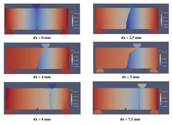
FIGURE 7. Displacement fields of cement paste specimens in three-point flexural test with an eccentric load dx.
