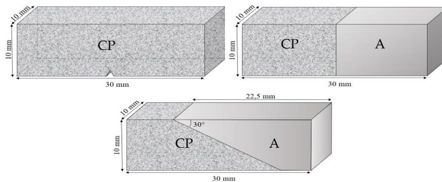
**FIGURE 1.** Specimens' geometries descriptions: cement paste (top left); straight aggregate composite with a  $90^\circ$  interface angle (top right); and  $30^\circ$  inclined aggregate composite (CP: Cement Paste and A: Aggregate).
