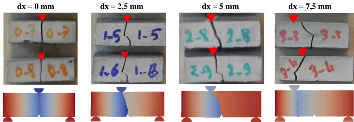
**FIGURE 11.** Results of cement paste specimens under three points bending with an eccentric load of  $dx$ : Top, experimentally (rupture profiles); Bottom, numerically (rupture profiles and displacement fields).
