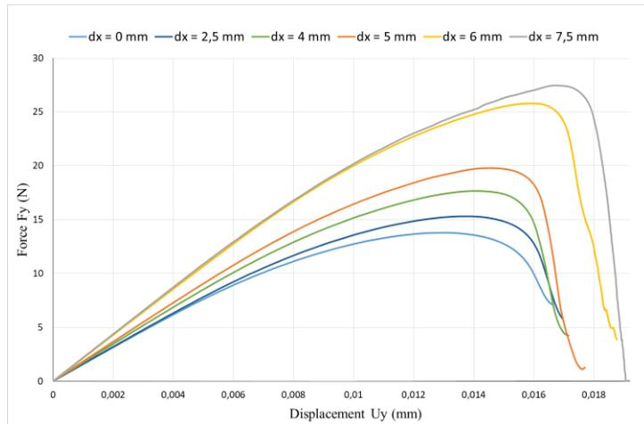
**FIGURE 8. Mechanical behaviors of cement paste specimens under non-symmetrical three-point bending tests ( $F_y$  : force applied vertically and  $U_y$  : displacement of the specimen in contact with the load application point).**
