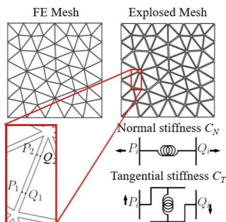
FIGURE 4. Illustration of the concept of the Volumic-Cohesive Finite Element Approach [5].
