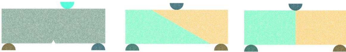
**FIGURE 6.** The cement paste mesh for the eccentric three-point bending test is shown on the left. Composite mesh for the centered three-point bending test with aggregate slanted at  $30^\circ$  in the center. Composite mesh with straight aggregate ( $90^\circ$ ) on the right.
