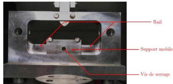
**FIGURE 2.** Design of the modular three-point flexion bench [3].
