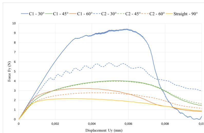
**FIGURE 10.** Mechanical behaviors of composite specimens under symmetrical three-point bending tests ( $F_y$  : force applied vertically and  $U_y$  : displacement of the specimen in contact with the load application point).
