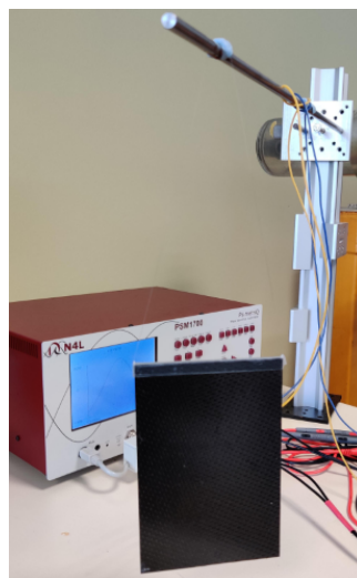
Figure 4 – Setup for the measure of C_0
