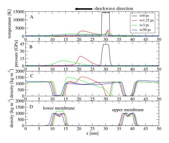
Figure 2. The profiles along the z-axis of the temperature (A), normal pressure component (B), mass density of water (C) and mass density of membrane (D) obtained at 0 ps (black), 1.25 ps (red), 3 ps (green) and 50 ps (blue). Shown are results obtained from the simulation of the normal membrane using a shockwave impulse I = 21 mPa.s and a 10 nm bubble.
