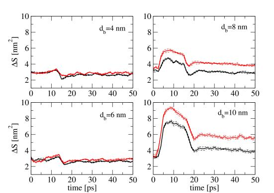
Figure 8. Time evolution of the pore area induced by the collapse of bubbles with different radius  $d_{\rm b}$  under a shockwave impulse I = 23 mPa.s. Show are results of the normal (black lines) and cancer (red lines) membranes. The average data (over 10 trajectories) are shown by the solid thick lines and the error bars are shown by the dashed lines.
