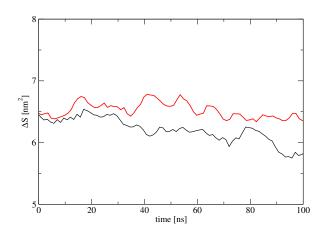
Figure 9. Time evolution of the pore area in the normal (black line) and cancer (red line) membranes under equilibrium condition at 300 K and 1 bar. The initial pores at t = 0 ns were perforated by a shockwave impulse of 25 mPa.s and a 10 nm bubble.
